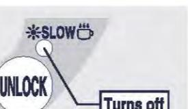
10 seconds after dispensing, the **UNLOCK** light turns off and the Automatic Dispense Lock is activated.
