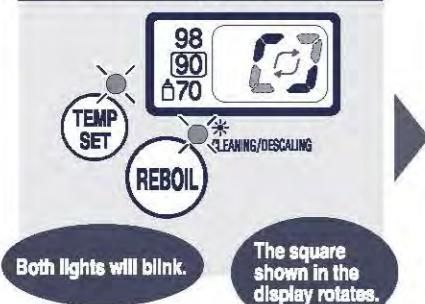
When the cleaning process is completed.
