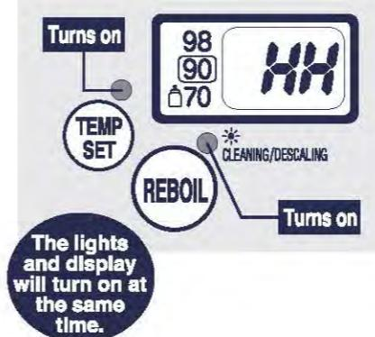
The Automatic Shut-Off function activates to shut down power to the heater in order to prevent damage from overheating. The Display will show "HH" to alert you that the Automatic Shut-Off has been activated. The following conditions may cause activation:
