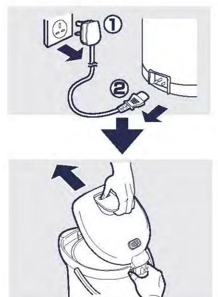
**2** Hold the product with both hands and dispose water where indicated "EMPTY FROM HERE" on the wall of the Inner Container.
